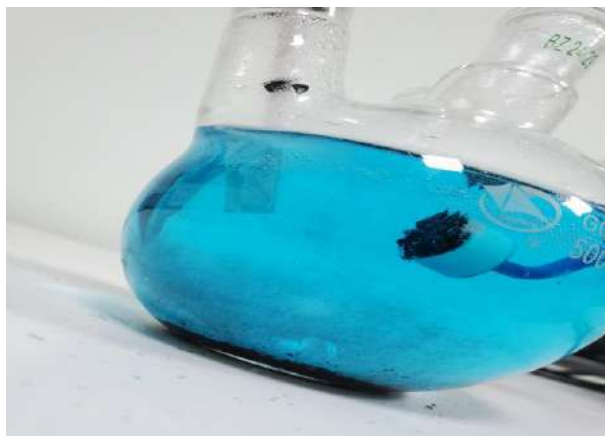
Figure 2(a). Copper powders formed on the cathode
