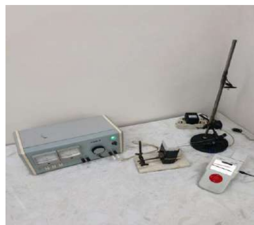
1-picture. Thermoelectric parameter measuring device for samples a) appearance of the measuring device b) measuring instruments
