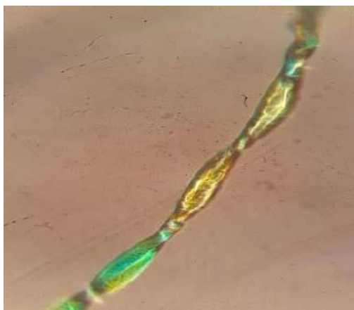
1-rasm. Yuvilmagan ingichka tolali “Surxon–104” navli paxta tolasining oq nur (A) ba qizil nur (B) ostidagi tasviri
