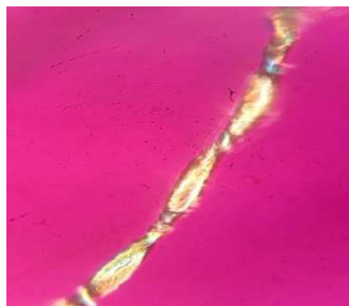
1-rasm. Yuvilmagan ingichka tolali “Surxon–104” navli paxta tolasining oq nur (A) ba qizil nur (B) ostidagi tasviri
