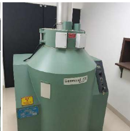
5-rasm. Gel-polimer elektrolit namunalarini Gammacell 220 Nordion International Inc. qurilmasida past dozali \text{Co} \gamma -nurlanish ta'sir qildirish.
