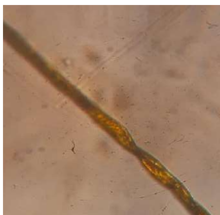
4 – rasm. Yod bilan legirlangan ingichka tolali “Surxon–104” navli paxta tolasining oq nur (A) ba qizil nur (B) ostidagi tasviri
