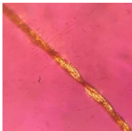
4 – rasm. Yod bilan legirlangan ingichka tolali “Surxon–104” navli paxta tolasining oq nur (A) ba qizil nur (B) ostidagi tasviri
