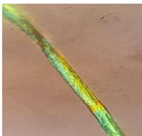
2–rasm. Yuvilgan ingichka tolali “Surxon–104” navli paxta tolasining oq nur (A) ba qizil nur (B) ostidagi tasviri
